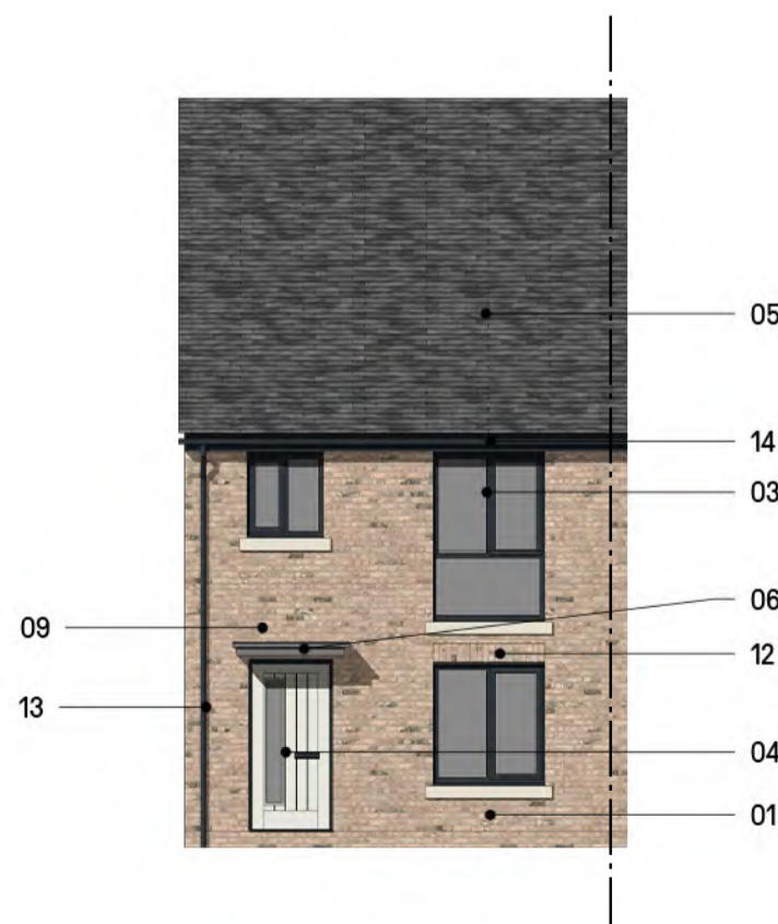
4 FRONT ELEVATION - A 1:100 APPLICABLE FOR PLOT 63 ONLY
